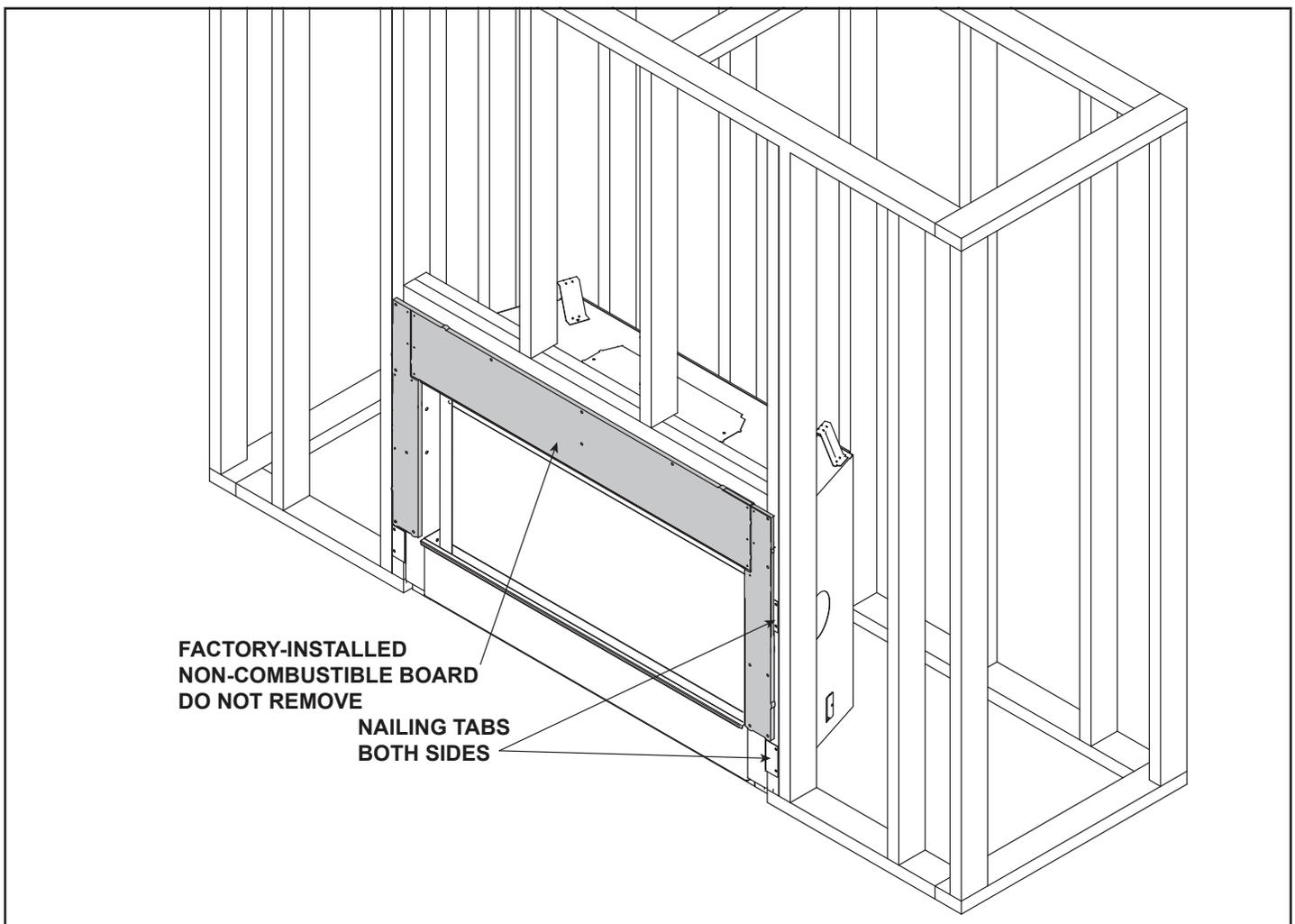
Figure 6.6 Proper Positioning, Leveling And Securing Of Appliance
