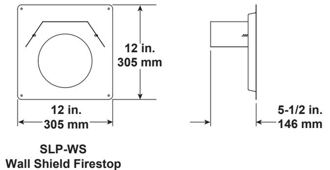
Figure 12.1 SLP Series Vent Components
