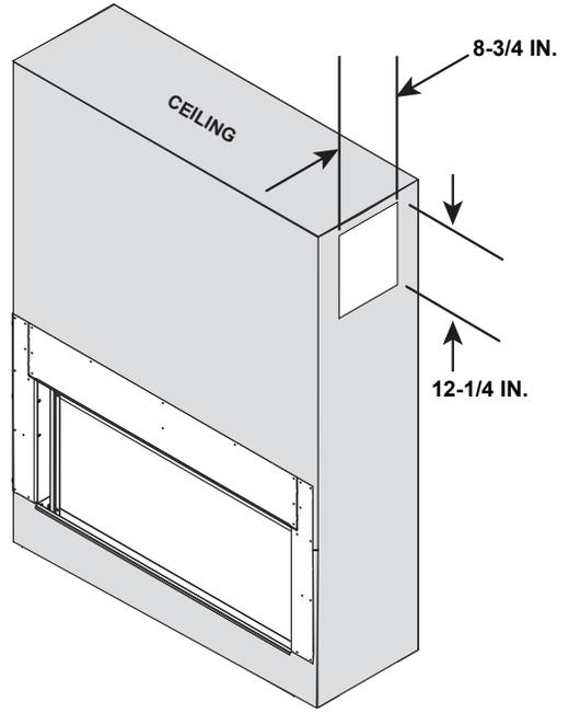
Figure 10.8 Finishing Material installed with Passive Heat Optional Heat Management System
