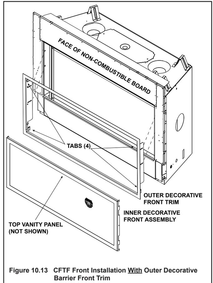
Figure 10.13 CFTF Front Installation With Outer Decorative Barrier Front Trim
