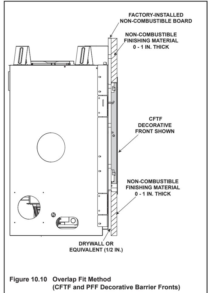
Figure 10.10 Overlap Fit Method (CFTF and PFF Decorative Barrier Fronts)
