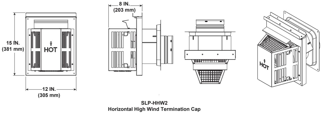
Figure 12.4 SLP series Vent Components
