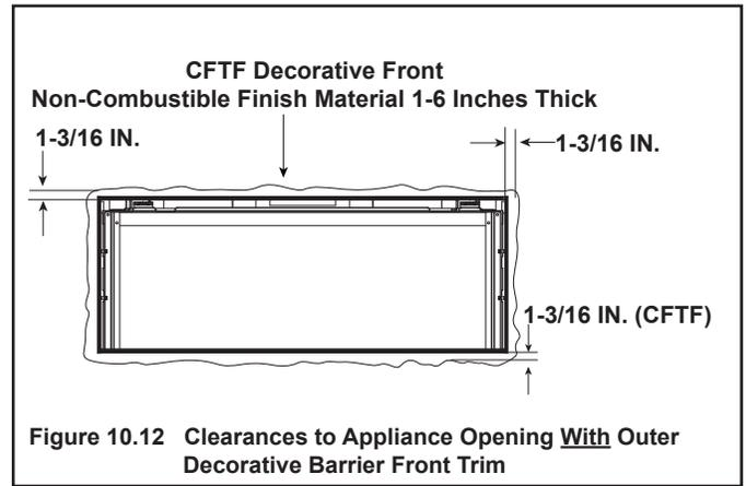
Figure 10.12 Clearances to Appliance Opening With Outer Decorative Barrier Front Trim
