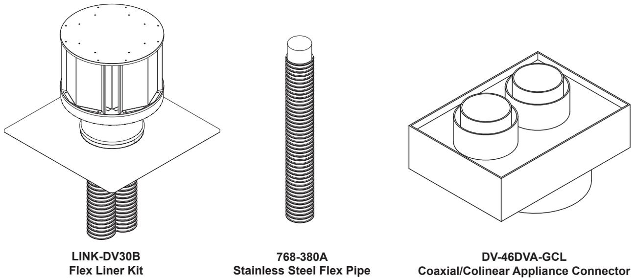
Figure 12.5 Coaxial to Colinear Vent Components
