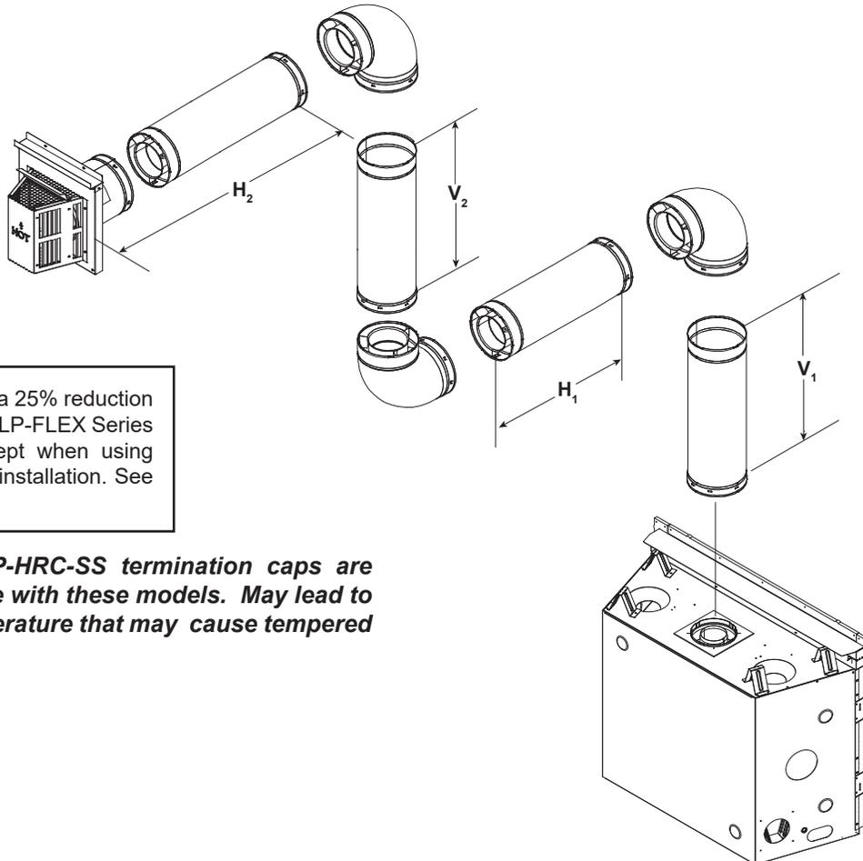
**Note:** There MUST be a 25% reduction in total H when using SLP-FLEX Series (6-5/8 inch) vent except when using the simple up and out installation. See Figure 4.10.
