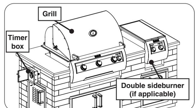
Fig. 11-3 Install grill, sideburner, and timer box
