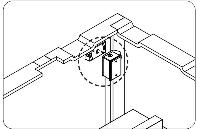
Fig. 9-2 Install electrical (as needed)
