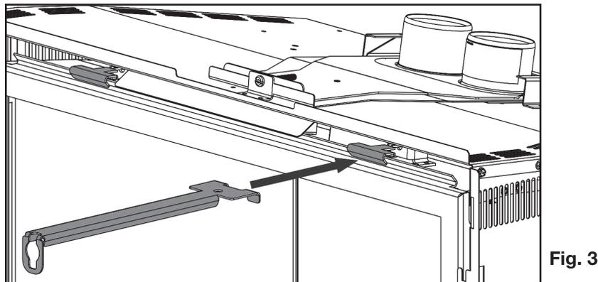
3. Reverse these steps to re-install the safety barrier and glass door. Ensure safety barrier is installed correctly.
