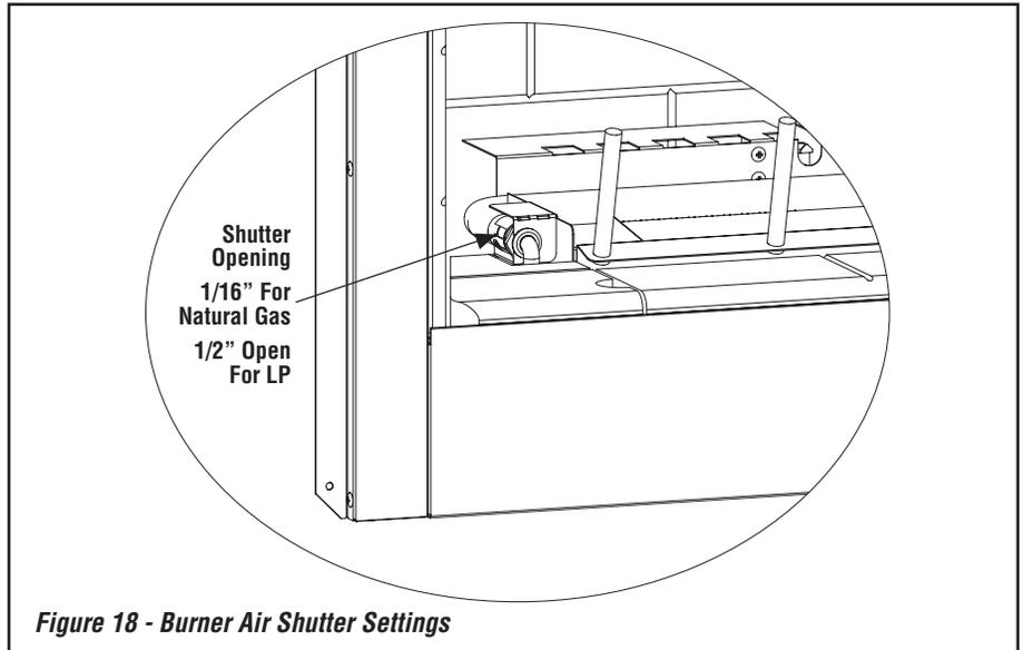
**Figure 18 - Burner Air Shutter Settings**
